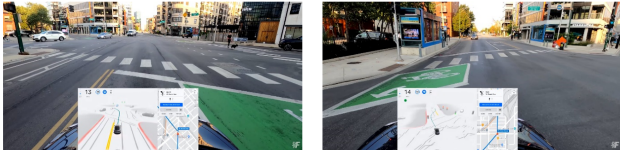
Fig. 1: Scene interpretation error. The vehicle control system is unable to correctly recognize the intersection indicated on the map and, as a result, enters the road to the left in the wrong direction. Images extracted from [9].
